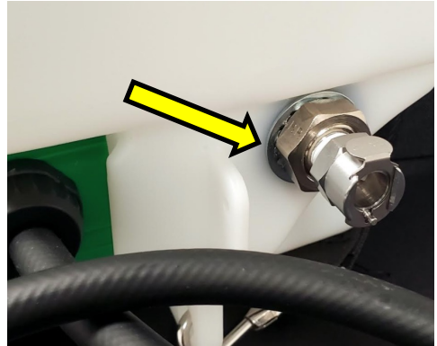
Bulkhead Drain Line Quick Disconnect
