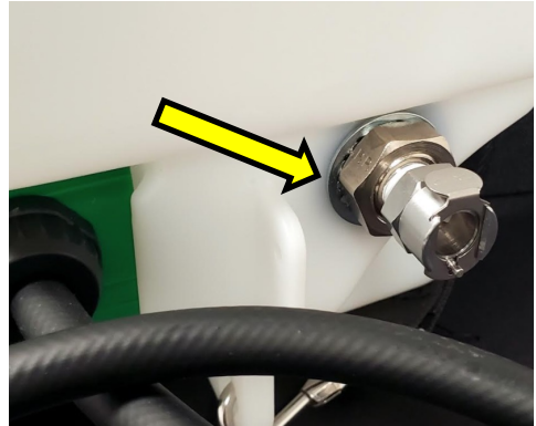
Bulkhead Drain Line Quick Disconnect
