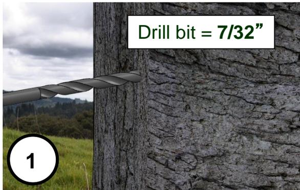
1. **Drill 1"** into sapwood (bark depth + 1") at slight downward angle.
