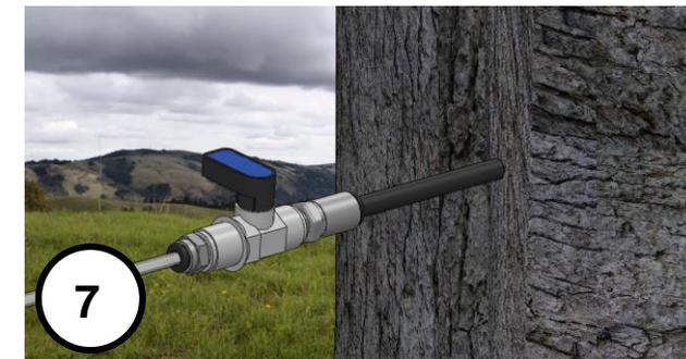
7. **Turn OFF** valve after tubing has emptied of product. Then wait 10-15 seconds before removing STINGER needle from drill hole.
