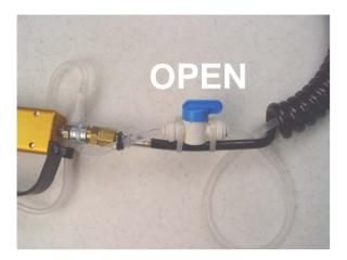
Make sure supply line valve is OPEN
