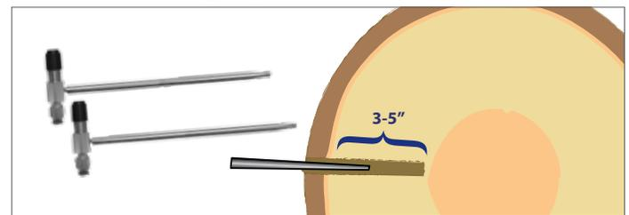
STINGER technology allows the applicator to apply products directly to palms without the use of an Arborplug. The STINGER needle is a high grade stainless steel which will provide many years of simple, reliable injection service. While the Arborplug is not necessary when using the STINGER needle, the Arborplug can be applied after the injection to seal the injection site.
